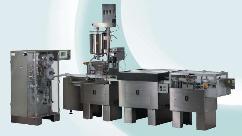
Modular line for the production of suppositories in thermoplastic cavities
